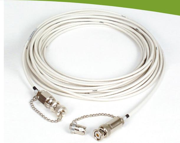
Triaxial BNC (bayonet) connectors are the 2-slot/lug, 1/4-turn locking type. The male connector has a pin insert and is always accompanied by a ferrule with locking slots. It is available only for cable mounting. The female connector has a socket insert and locking lugs that mate with the ferrule. It is available for cable mounting or panel (bulkhead) mounting, with either flange or threaded mounting.
