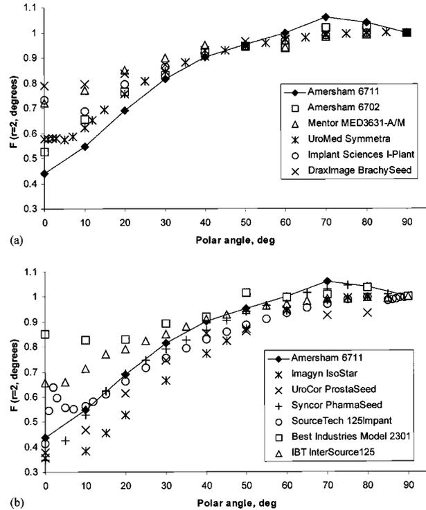
FIG. 4. Anisotropy Function  $F(r, \theta)$ ; (a) Anisotropy Functions for the sources with the radioactivity adsorbed onto the internal core of the source for a radius of 2 cm, (b) Anisotropy Functions for the sources with the radioactivity adsorbed onto the internal core of the source for a radius of 2 cm.
