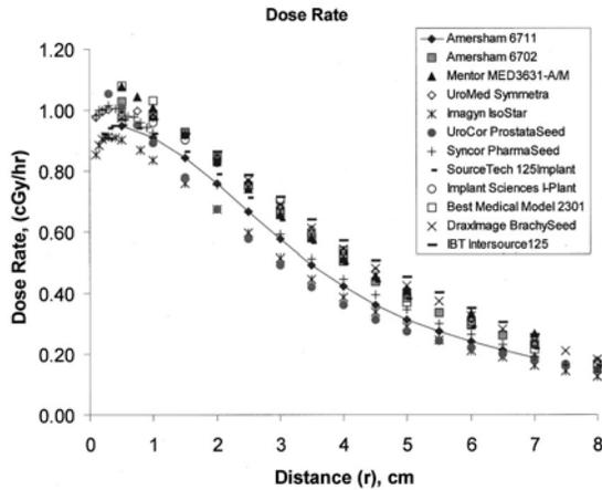
FIG. 5. Dose Rate Values for source strength of 1 U.
