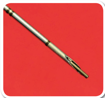
Loose Seed Loaded into Localization Needle
