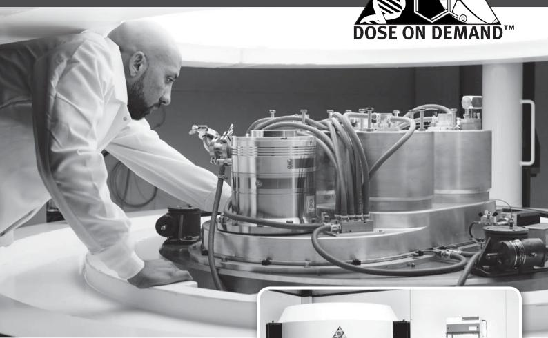
The BG-75 Biomarker Generator integrates a compact mini-cyclotron, kit based micro-chemistry, and automated quality control, simplifying in-house production of <sup>18</sup>F-FDG and advanced biomarkers.
