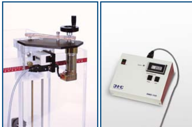
Left: Motor drive assembled to the depth drive Right: Remote control/display module
